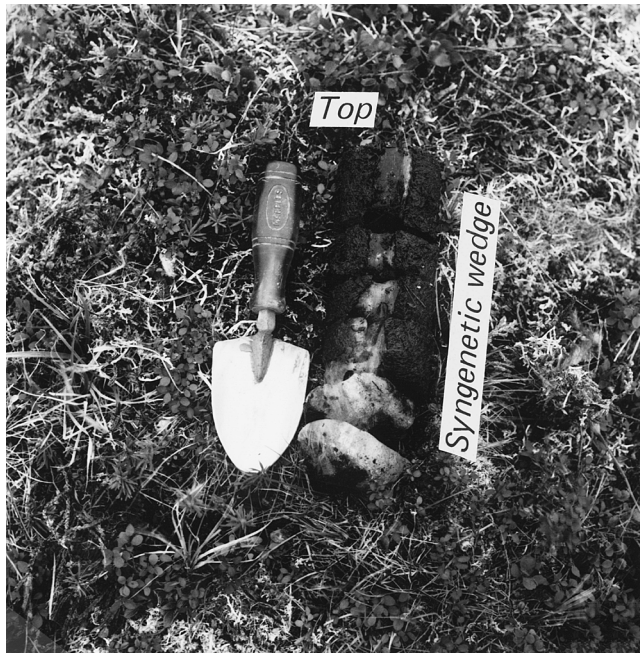
FIGURE 34. Drill core collected at the drilling site of Figure 33 showing the top of a narrow syngenetic wedge that propagated upward from the epigenetic wedge at the bottom. The 20 cm long trowel provides scale.
