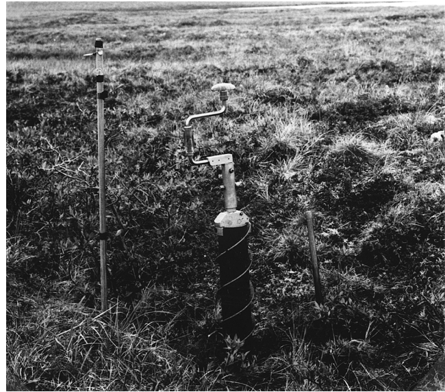
FIGURE 33. Photo of a drilling unit that was being used to collect a frozen core in an ice-wedge trough where, in the 1967 to 1987 period, winter observations showed that the wedge cracked 15 times along the same line at the frozen surface of the ice-wedge trough (Mackay, 1992b, Fig. 6, site 60).
