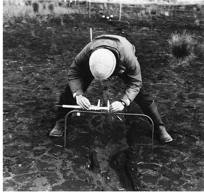
FIGURE 41. The photograph shows the ice-wedge trough of a crack that opened in the second winter (1979/80) following lake drainage at Illisarvik. The change in separation across the ice-wedge trough, from the previous measurement, was being measured with an "arch" type of crackmeter where the two vertical supports were inserted only into the active layer. The separation being measured was for crackmeter #85 (see Fig. 42).
