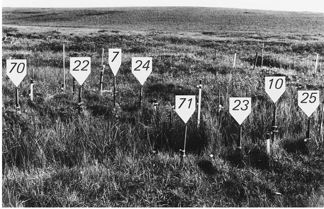
FIGURE 27. Photograph of four pairs of bench marks of different lengths installed at different depths on the polygon ridges between Polygon A and Polygon B (See Fig. 20 for locations).
