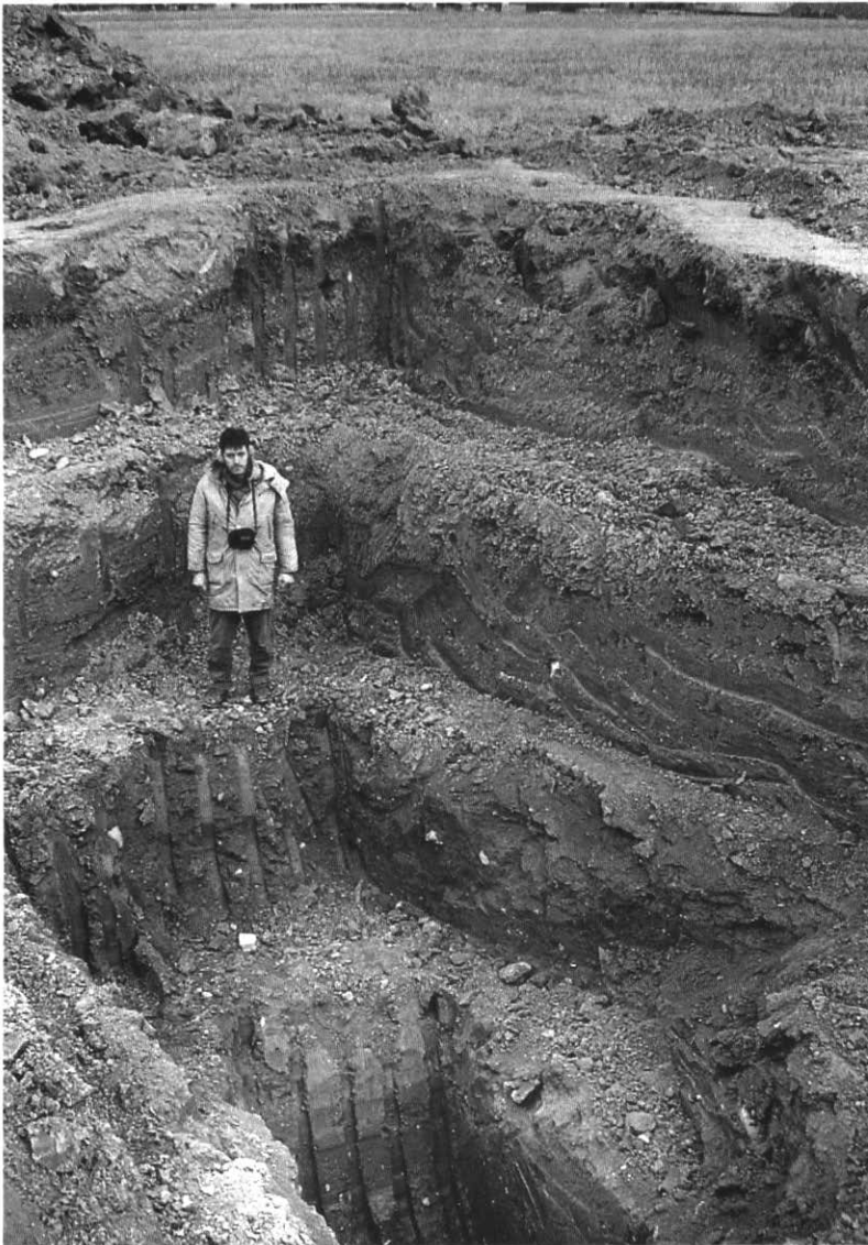
Figure 13 Test pit through Halton Till.
