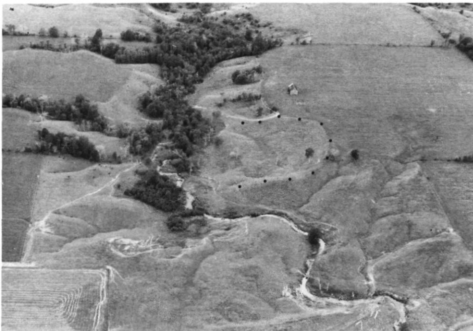
FIGURE 10. Photograph of area immediately upstream of 1979 Mabel slide showing small scar (dotted) on north (right) valley side ( R/H = 3 ) characteristic of the Lachute region.
