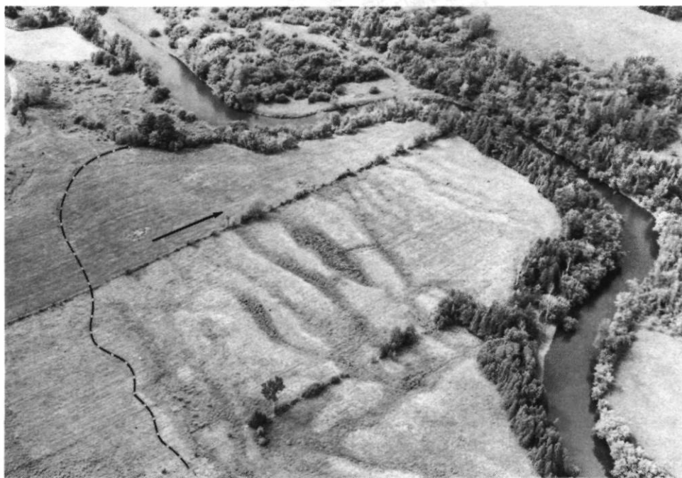
FIGURE 3. Air photograph of flowbowl (West Lachute (H)). Note well-defined "ribbed" microrelief, and full translation of spoil across valley.
