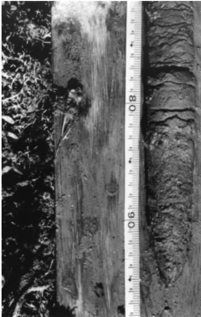
FIGURE 11. Stratigraphic contact between lensed clay and sand at the base of a core in the plateau.
