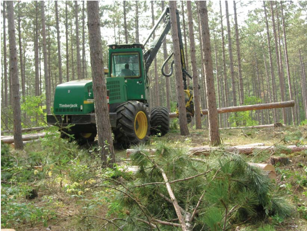
Figure 1. A tree harvester used in this trial for thinning red pines at the York site.
