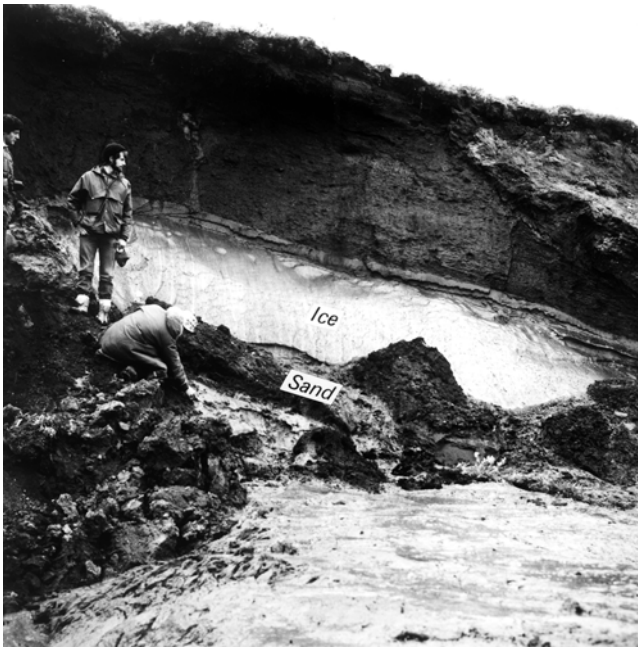
FIGURE 64. Photograph of Pingo 21 (Whitefish Summit Pingo) taken in 1973. The exposed section, from the ground surface downward, was: 3.5 m of a stony clay; 0.35 m of fine sand; 3 m of nearly pure ice; and frozen sands to the bottom of the exposure.
