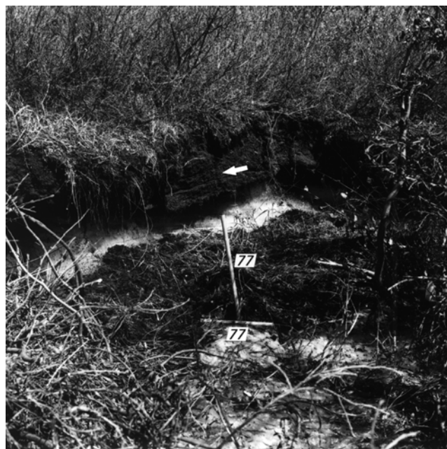
FIGURE 54. BM 77 (Fig. 53b) broken by the growth of 0.75 m of intrusive ice in the winter of 1975/76 as a result of renewed normal faulting along "dilation crack x" (Fig. 40). The arrow points to the location where the top of BM 77 was broken off. The broken top is labelled "77" and is horizontal at the bottom of BM 77. The water source was along the fault as shown in Figure 55.
