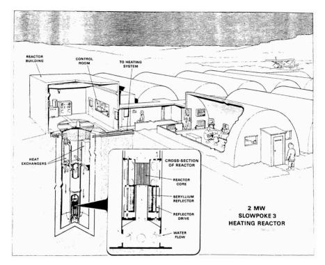
Figure 2. 2MW Slowpoke-3 Heating Reactor.
