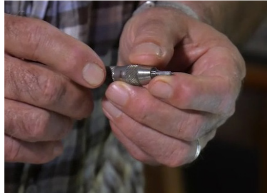
A carbide-tipped scribe used by Pierre Hébert to scratch his drawings onto black film stock. See database entry.
