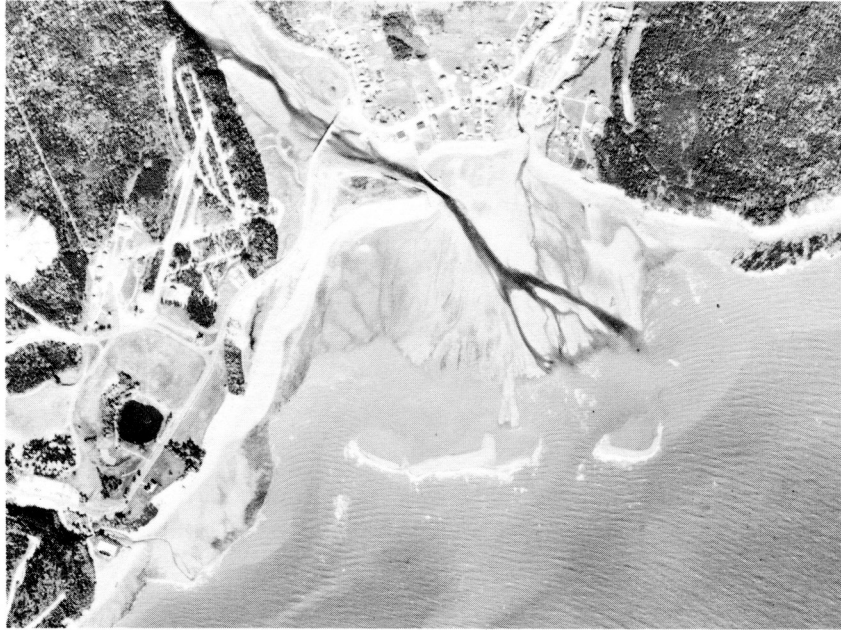
Figure 1. Alma River delta near low tide: aerial photograph, 1959. Note the straight distributary channels, the abandoned distributary tongue, and the geniculate bars with new deposition opposite the tongue. A bedrock abrasion platform is seen at extreme right beneath cliffs. North is at the top of the photograph, and the width of the area shown is about 7000 feet.
