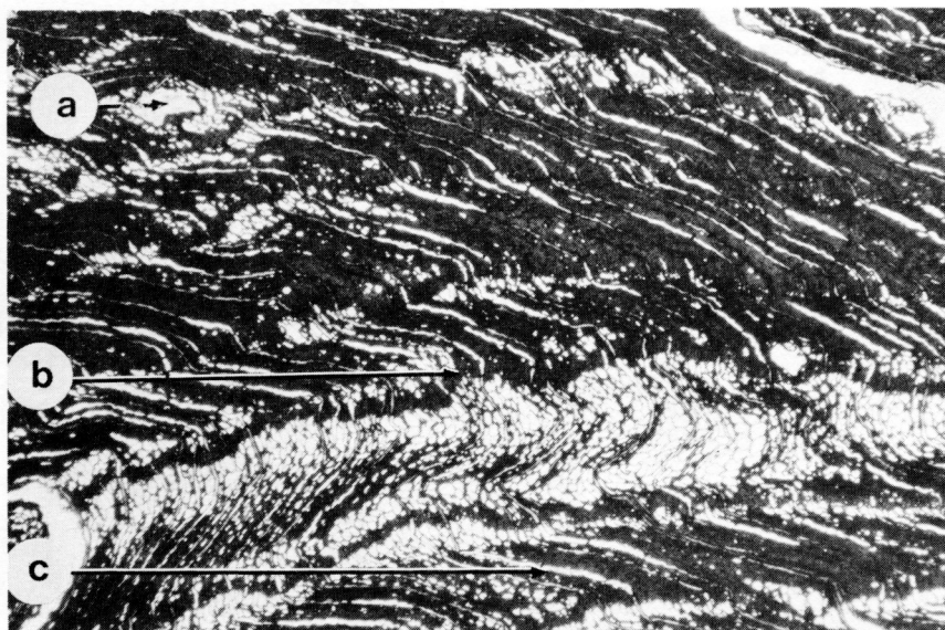
Fig. 1. Wood Specimen No. 1. Low power view of collapsed wood. (50X)
