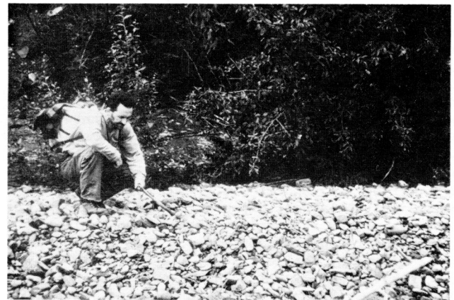
FIG. 3 Well sorted, imbricated river gravels occurring a few miles downstream from a fall line in northeastern British Columbia. Mean diameter of cobbles is about 100 mm. Hand-held hammer is parallel with fabric direction; this fabric is an example of sedimentary anisotropy.
