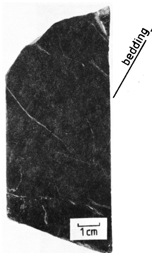
Figure 15 - Core sample of conformable galena and sphalerite (grey) in black slate. Small cross-cutting veinlets contain sphalerite. The section that includes this sample assayed 2.24 % Pb and 5.36 % Zn.
