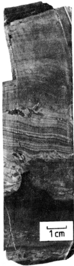
Figure 10 - Quartz metawacke interbed in black slate. Plane lamination and load casts on the basal contact of the beds are features of many interbeds in the Halifax Formation. Pyrrhotite in small pods and in cubic habit (after pyrite) disrupts the bedding.
