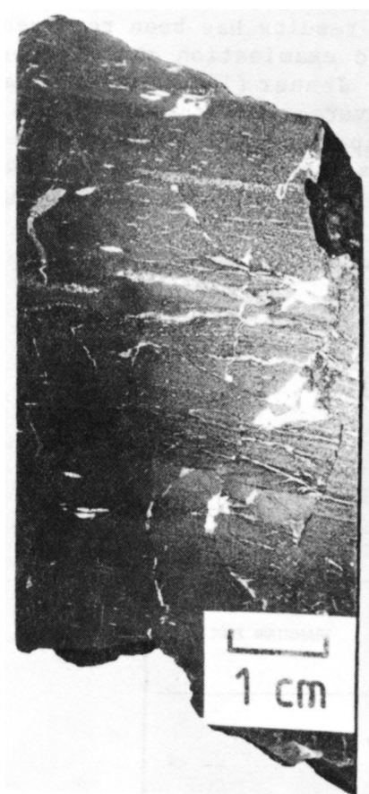
Figure 17 - Discontinuous sphalerite and galena veinlets and adjacent disseminations in black slate.
