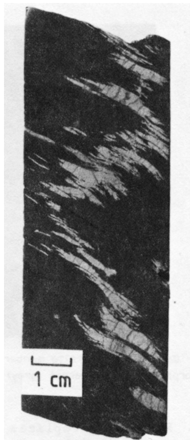
Figure 16 - Transposition of a pyrrhotite bed along the cleavage in the Halifax Formation. The sulphide bed is at a high angle to the cleavage and parallel to the drill core at this location.
