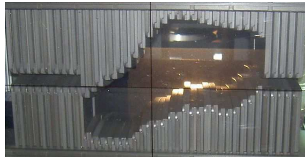
Fig. 1. The leaf pairs of a multileaf collimator (MLC)
