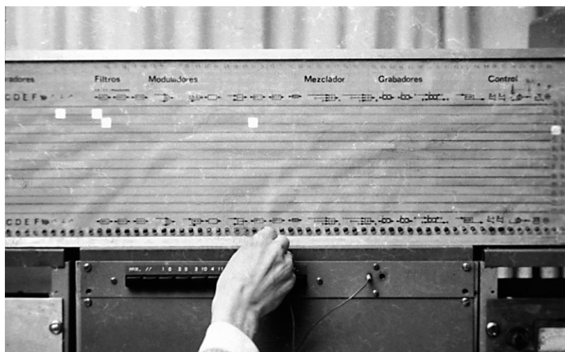
CLAEM – Instituto Torcuato Di Tella, Buenos Aires, Argentine, 1966. Touch-controlled patch-bay, designed by Fernando von Reichenbach, built with spare part from the telephone company (Collection de musique électroacoustique latino-américaine, Fondation Daniel Langlois).
