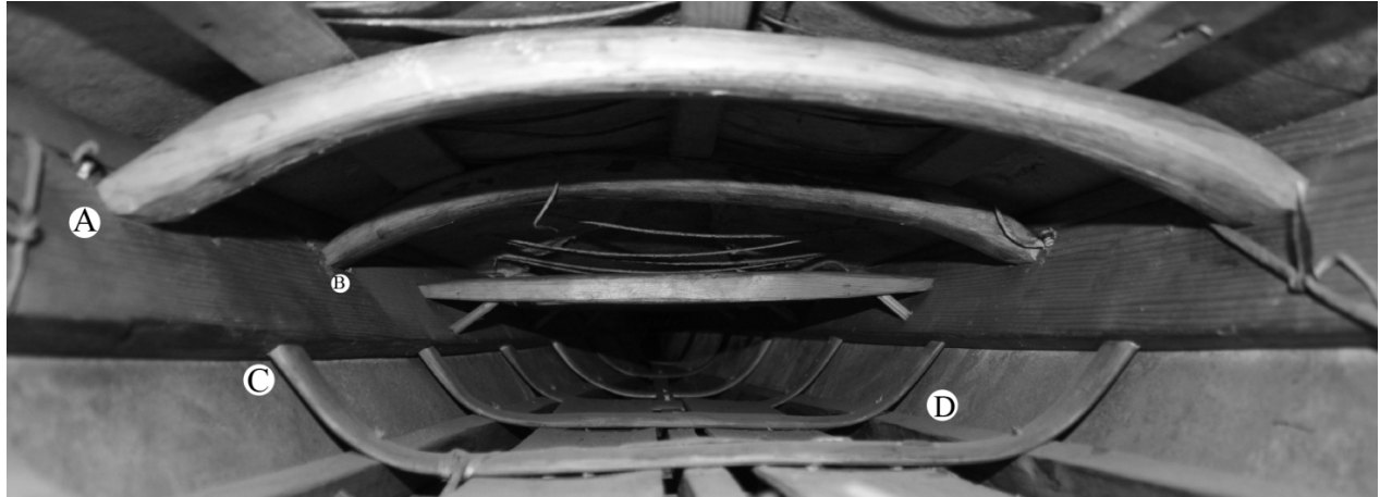
Figure 6. Interior of a Greenlandic kayak: a) cambered crosspiece mortised securely to the gunwale; b) cambered crosspiece mortised securely to the gunwale; c) ribs mortised to the gunwale; d) stringer held in position by the ribs. Photo: courtesy of the Danish National Museum, item Lc. 148, photographer: Matthew Walls.
