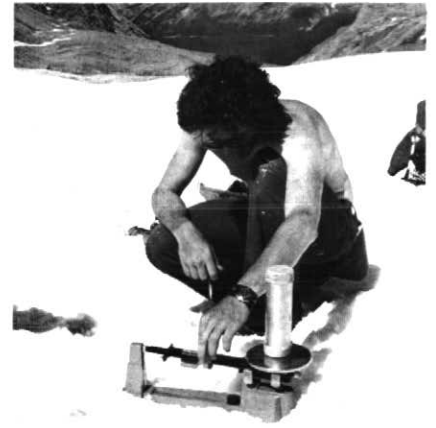
Figure 1 Snow density determination, Peyto Glacier.
