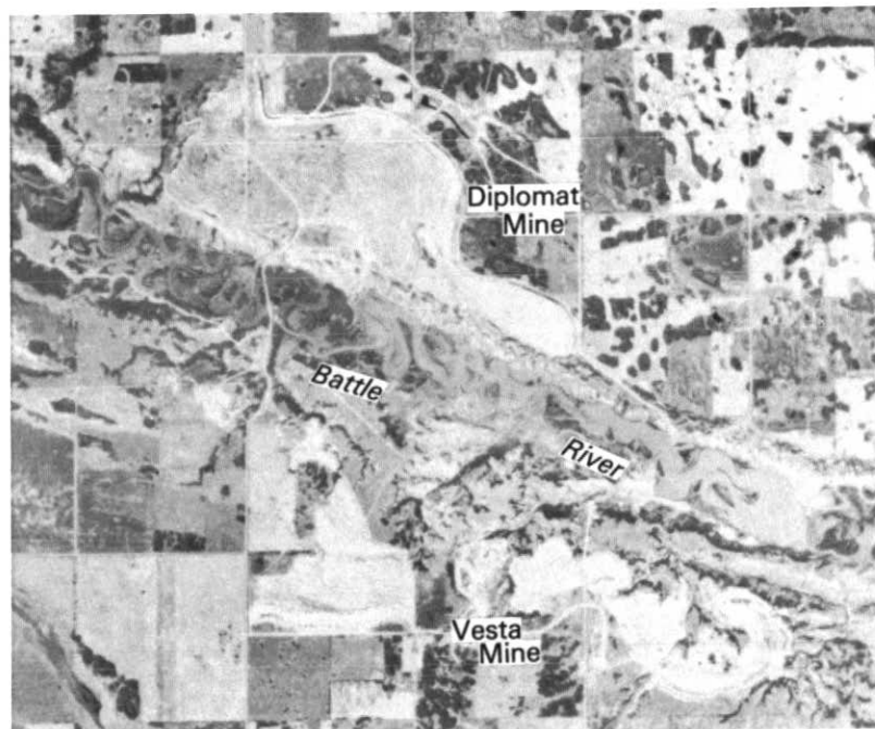
Figure 17 Aerial photograph of the Vesta and Diplomat coal mines along the Battle River near Forestburg (Fig. 14). The Plains Hydrology and Reclamation Project features extensive instrumentation of both the mine spoil (light-tones, ribbed areas) and adjacent undisturbed
