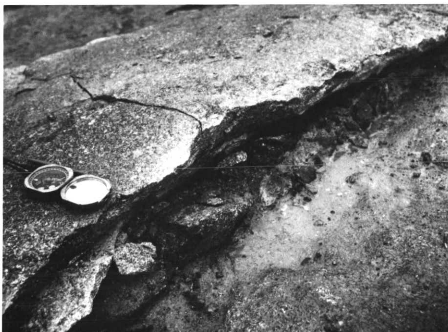
Figure 7 View of pop-up induced by removing till overburden. Note axial crack, gap under buckled slab, and dirt piled up against former
