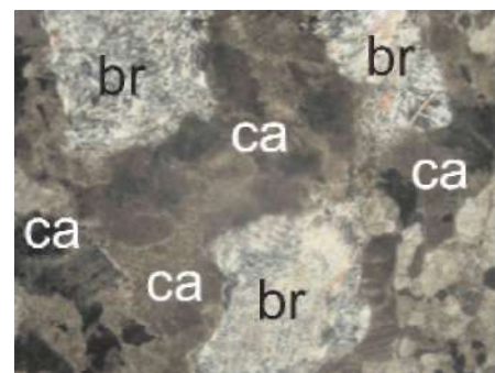
Figure 7. Photomicrograph of brucite (br) aggregates in carbonate matrix (brown). Matrix consists predominantly of calcite (ca). Field of view approximately 2.5 mm, plane light.
