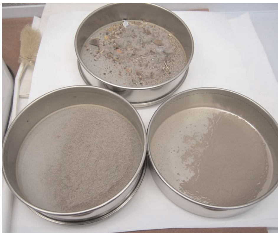
Figure 4. In residential surveys, house dust is collected using a vacuum sampler and is then air-dried and sieved to appropriate size fractions. Large particles such as coins and pet hair (top) are separated from the sieved fractions used for chemical analysis (less than 80 micron fraction, bottom right) and mineralogical characterization (80 to 150 micron fraction, bottom left). From Rasmussen et al. (2007b).
