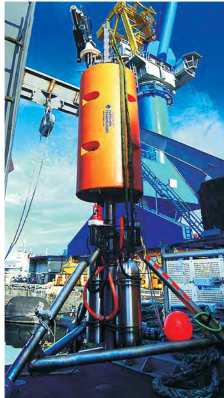
Figure 7. COVIS multibeam sonar, used to obtain 3D images of 3D hydrothermal vent fluxes, prior to deployment at the Endeavour Segment of the Juan de Fuca Ridge (2300 m water depth).
