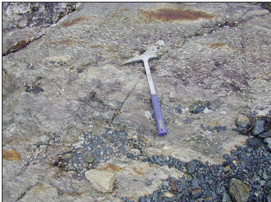
Figure 1. Reworked quartz-feldspar crystal tuff of the Nepisiguit Falls Formation, Brunswick No. 6 mine.
