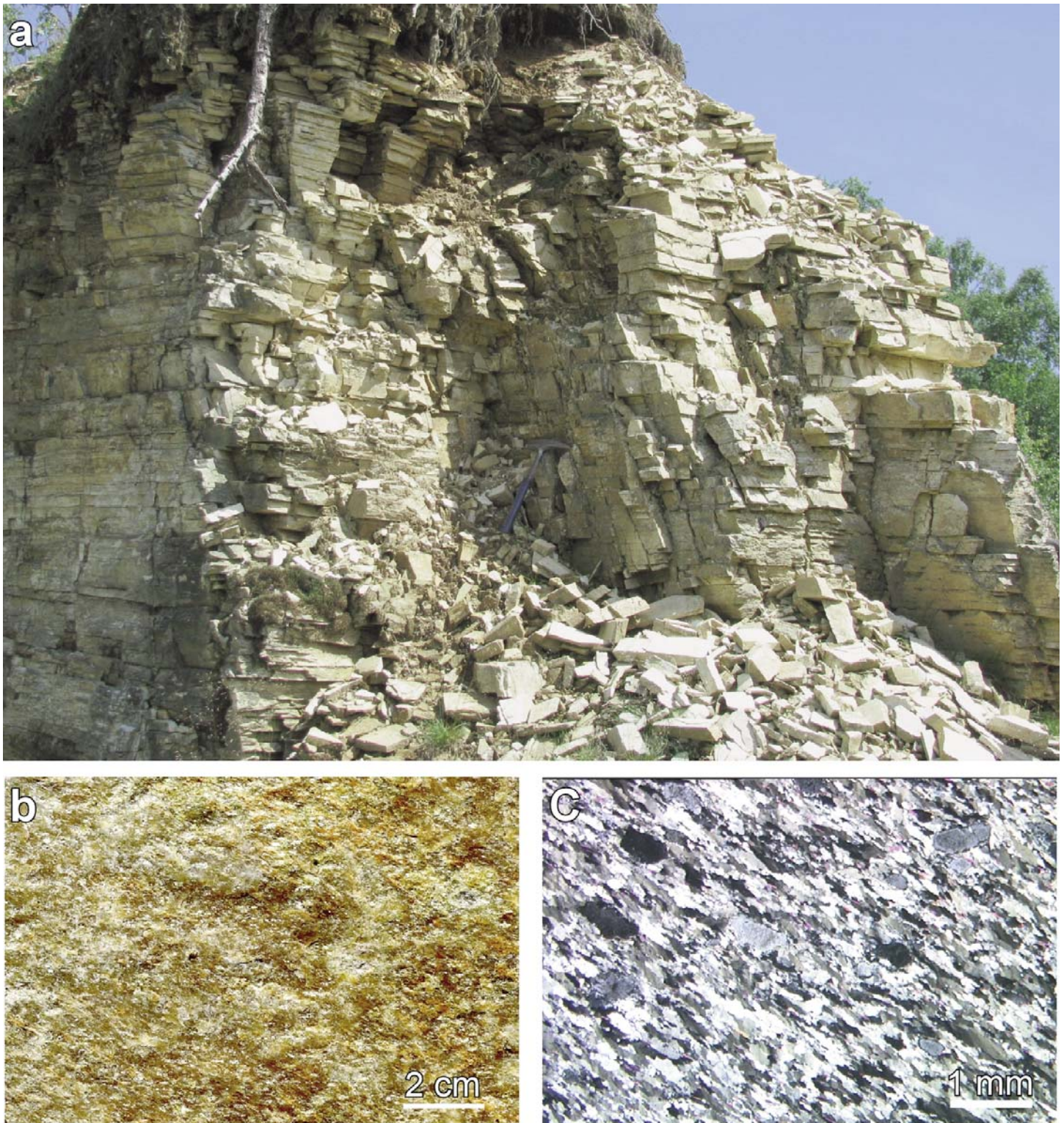
Figure 8. Bargiolina Quartzite: a) Quarry site located on Mount Bracco (site 15 in Figure 2); b) macroscopic aspect of the rock, characterized by a natural split surface defined by thin mica layers; c) microscopic aspect (crossed-polarized light), marked by a strong dimensional preferential orientation of quartz crystals.
