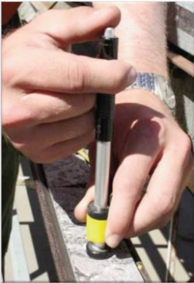
Figure 5. Left: example of hand-held measurement of drill core sonic velocity. Right: example of a Geotek multi-sensor core logger used for collecting petrophysical measurements (e.g. gamma density, p -wave velocity, resistivity, magnetic susceptibility, etc.) from drill core.
