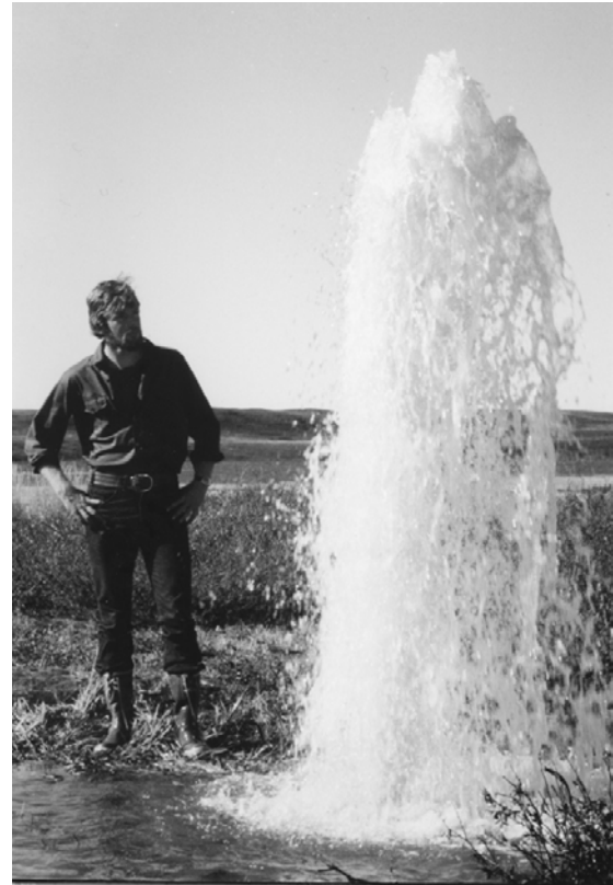
FIGURE 5. Drill-hole flow from Pingo 14 in 1976 (see Figs. 35 and 36 for location). The gusher that rose to a maximum height of 2.6 m issued from a 7.5 cm diameter hole from a depth of 22 m. The water temperature was about -0.1^{\circ}\text{C} (Mackay, 1979).
