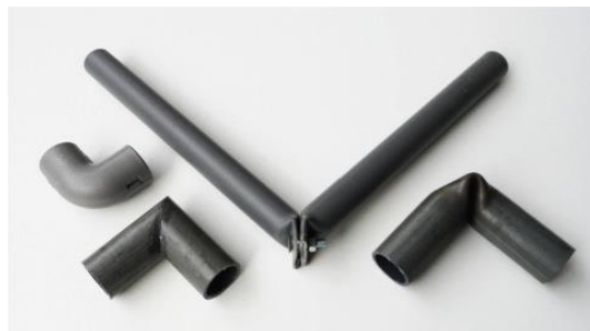
Figure 5. Alternative ways to create a 90° joint, listed by Modular vegetable protection cage projects.
