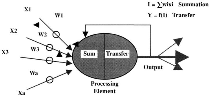
Note that various inputs to the network are represented by the mathematical symbol,  $x(n)$ . Each of these inputs is multiplied by a connection weights  $w(n)$ . In the simplest case, these products are simply summed, fed through a transfer function to generate a result, and then output. Even though all artificial neural networks are constructed from this basic building block the fundamentals vary in these building blocks and there are some differences.
