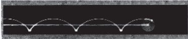
6-33. Path of a point on the rim of a rolling wheel. This curve, a cycloid, shows the path as it appears to an observer standing alongside. One small light was mounted on the rim of a wheel, and another light at the center. The camera shutter was held open while the wheel rolled.
