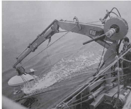
Figure 3. A hydraulic crane is used to lower and raise the CECS towed body, which contains the echo sounder's transducer, as part of the acoustic fish-counting program. BIO, Biennial Review 1973/74, 242.
