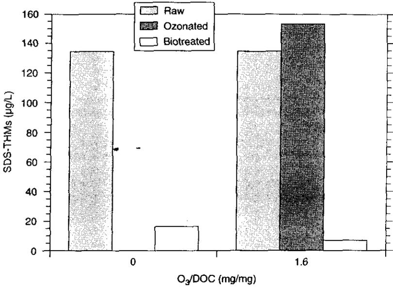
**Figure 7** Formation of trihalomethanes under simulated distribution system conditions.
