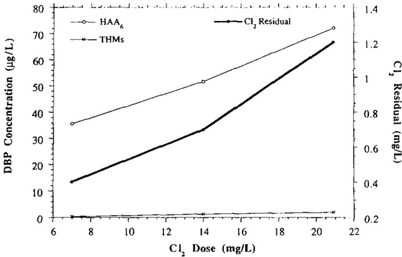
**Figure 10** Breakpoint chlorination curve for biotreated effluent (DOC = 6.9 mg/L; NH<sub>3</sub>-N = 1.84 mg/L). DBP = disinfection by-products.
