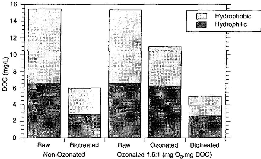
**Figure 5** Fractionation of DOC (< 1  $\mu$ m) on XAD-8 resin: effect of biotreatment and ozonation.
