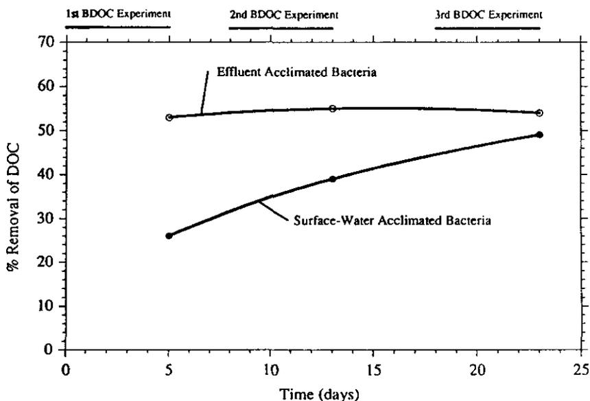
**Figure 1** Successive BDOC cycles using surface-water-acclimated bacteria or effluent-acclimated bacteria.
