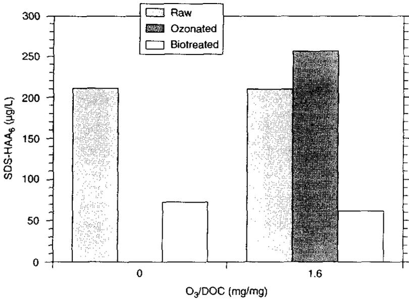
**Figure 8** Formation of haloacetic acids (HAA<sub>6</sub>) under simulated distribution system conditions.
