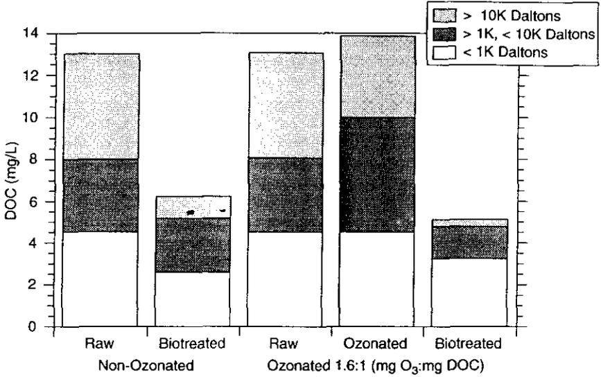
**Figure 4** Fractionation of DOC (< 0.45  $\mu$ m) by subsequent ultrafiltration: effect of biotreatment and ozonation.
