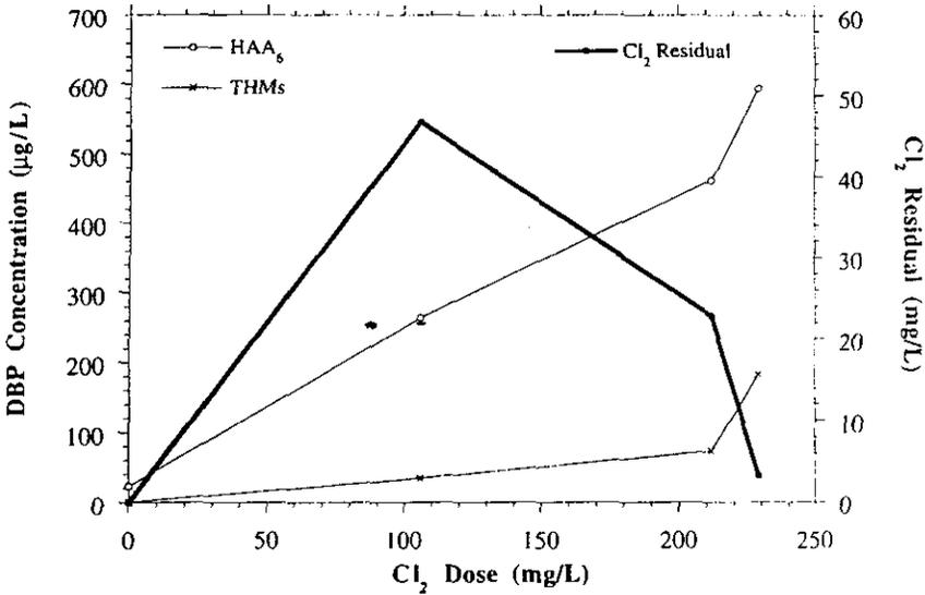
**Figure 9** Breakpoint chlorination curve for raw effluent (TOC = 16.1 mg/L; NH<sub>3</sub>-N = 27.9 mg/L). DBP = disinfection by-products.
