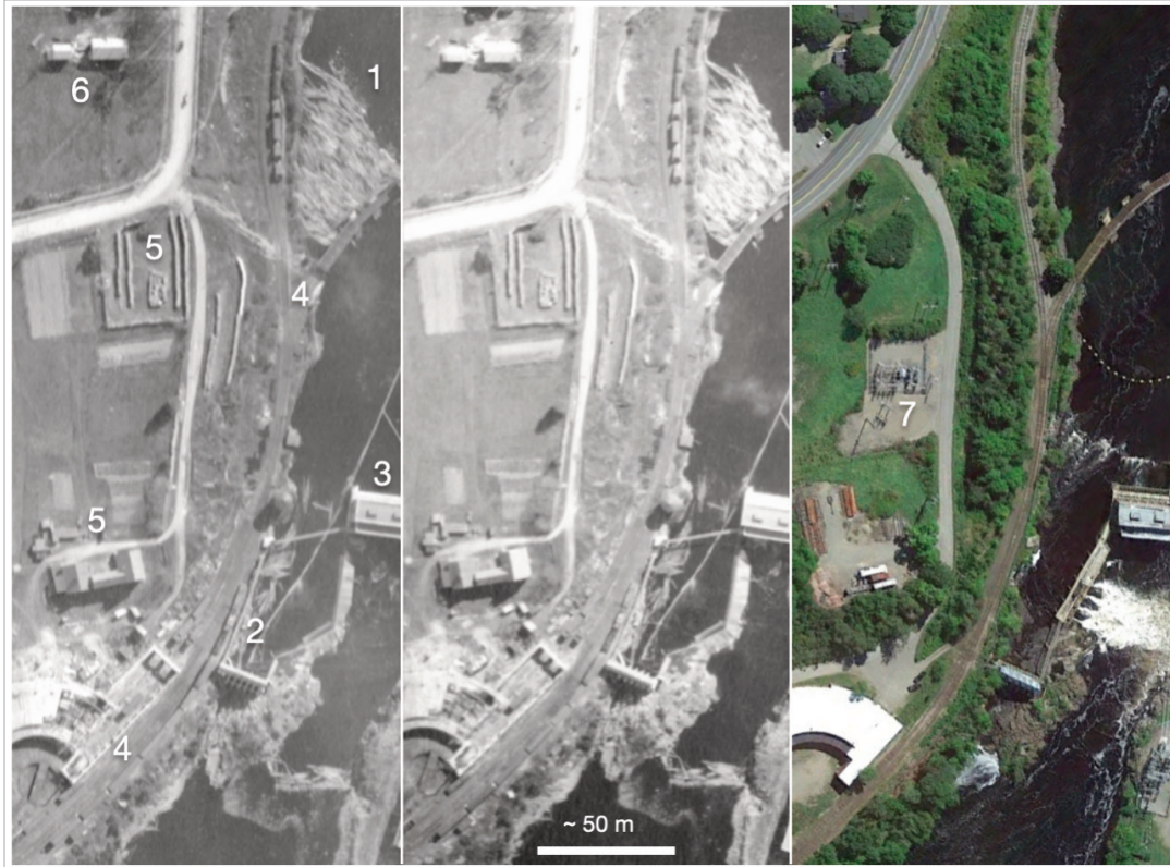
Figure 6. Stereopair of 1921 aerial photographs (left, centre) displaying a heavily industrialized section of the St Croix River near Union Mills, with log rafts (1), log booms and spillways (2), power generating facilities (3), railroad network and roundhouse construction (4), lumber yard (5) and lumber storage piles, and rural farmstead (8). The colour image (right) shows the same area in 2015; power generating facilities are still in place, with the addition of a transformer station (7). Source: NAPL (1921 air photos K3-7, K3-8) and IBC – Geo.NB (2015 colour image).
