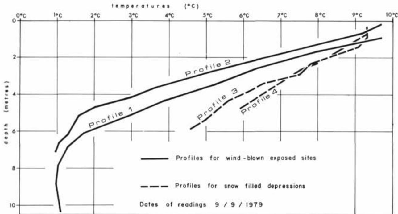
FIGURE 20. Temperature profiles for four old drill-holes at 1000 m in the col between the south and north summits of Mont Albert.
