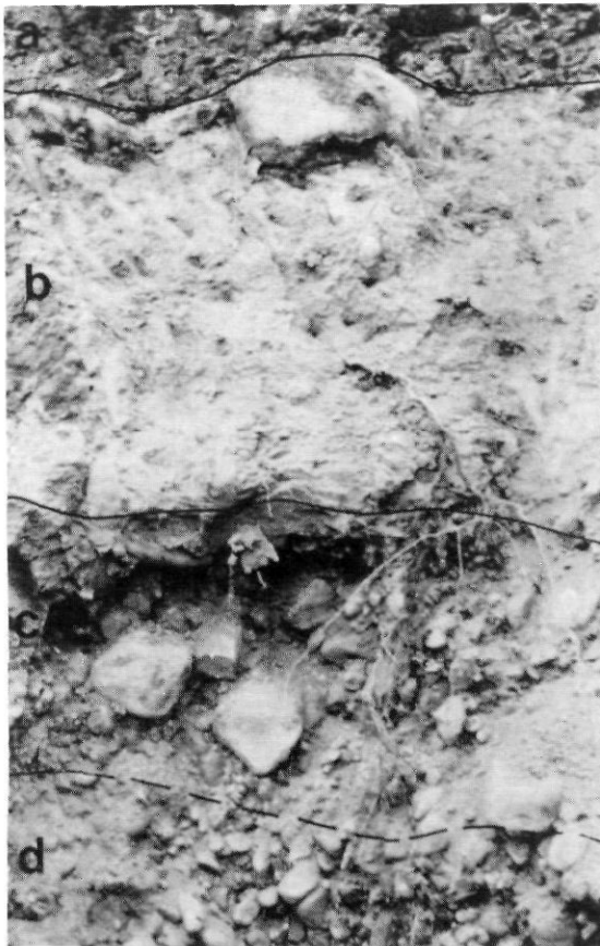
FIGURE 10. Top of Mountain River section: a) glaciolacustrine deposit; b) 50 cm of loess; c) paleosol in gravels; d) gravel parental material.
