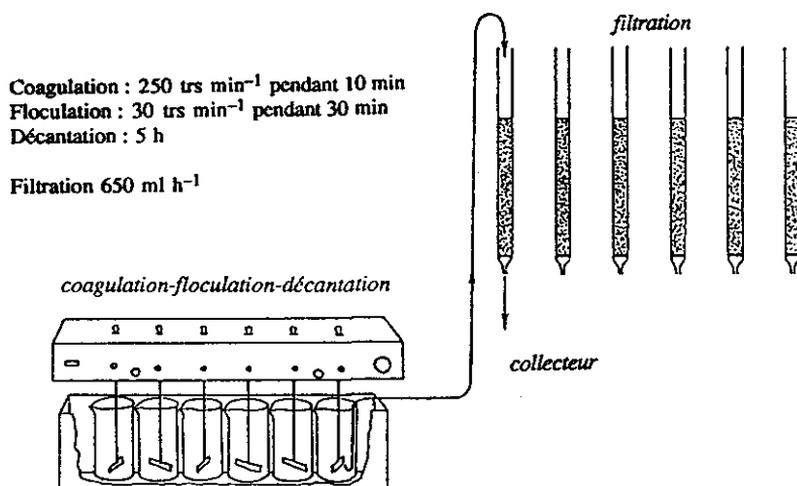
Figure 1 Méthode de coagulation-floculation-clarification.
