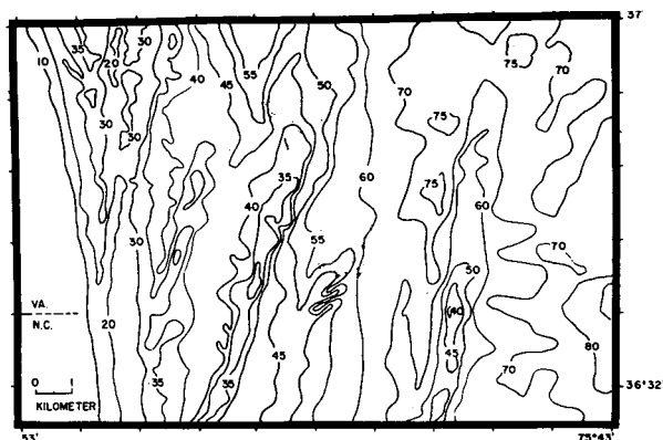
Figure 6 – Bathymetry of False Cape Study area, from 1922 US C&GS survey. Depth in feet.
