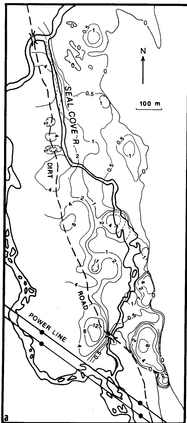
Fig. 3. a) contoured overburden thicknesses from combined data; b) contoured buried granite surface as elevations above sea level in meters. NOTE: all contours in meters; contour intervals are variable.
