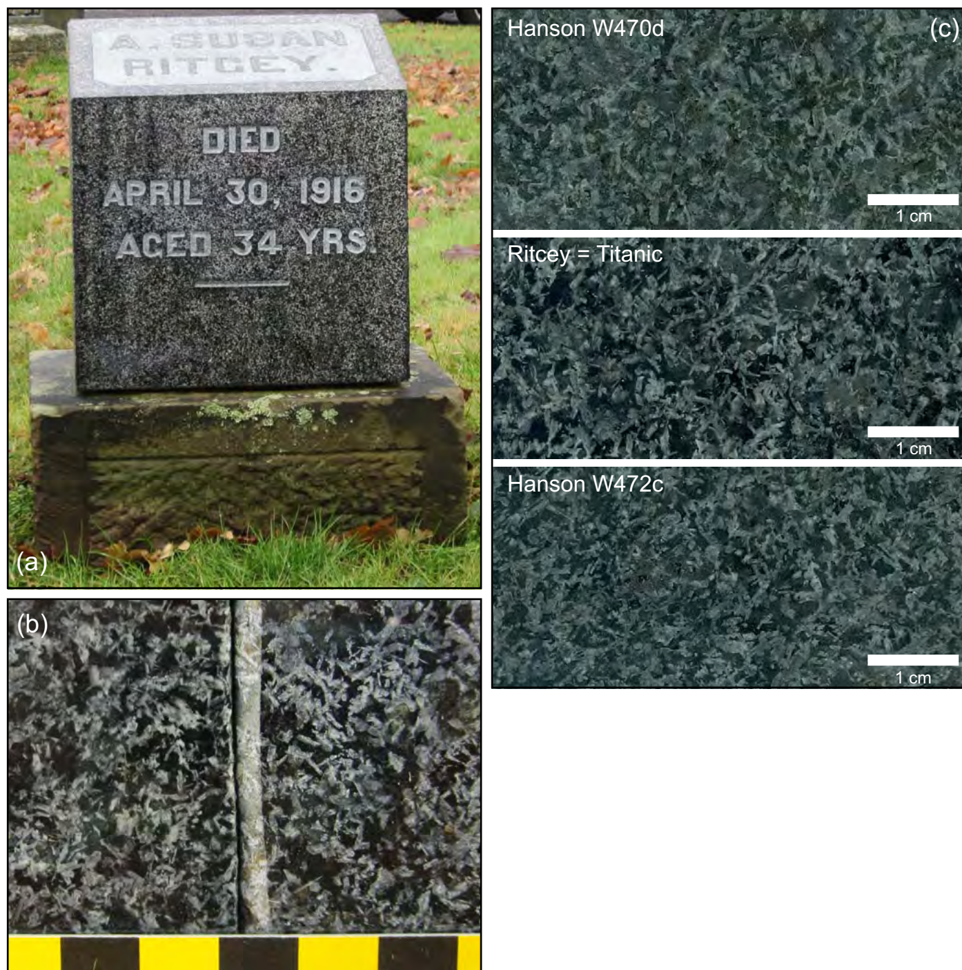
Figure 2. Macroscopic comparisons of the Ritcey headstone, Titanic headstone, and Hanson quarry. (a) Headstone of A. Susan Ritcey (1916) is the same size, and has the same chisel shape, as many of the Titanic headstones. The importance of the Ritcey headstone was to provide a second sample of Titanic material. (b) Ritcey headstone (right) has the same “snowflake” texture as the Baxter headstone (left). Scale division are in cm. (c) Textural comparison of the Ritcey headstone and two samples from the Hanson quarry.
