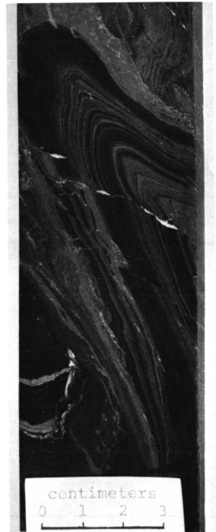
Figure 1 Specimens of laminated ore from sedimentary-type stratiform ore deposits: a) laminated sulphide and chert, from Mt. Isa, Australia; b) laminated argillite with sulphides, from the Sullivan deposit, Canada; c) laminated sulphide and darker chert, from the Howards Pass deposits, Canada.
