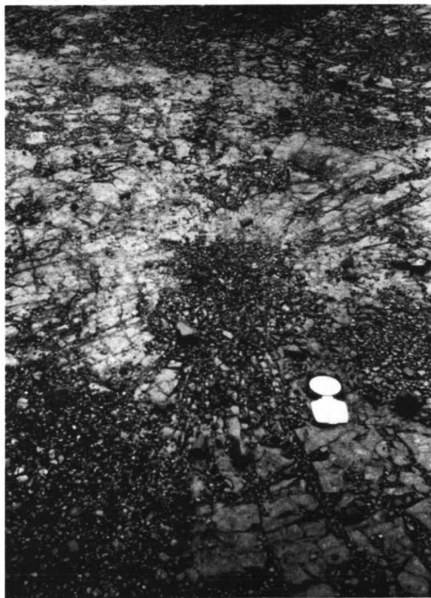
Figure 12 Fractures radiating out from a small explosion crater on the floor of McFarlane Quarry, near Ottawa, Ontario. The major population of fractures is aligned parallel to the open Brunton compass and clusters close to the azimuth of S_{Hmax} as defined by other criteria in the region.
