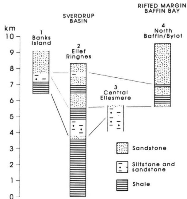
**Figure 11** Generalized stratigraphic columns showing thickness variations and geologic correlations of Mesozoic and Cenozoic strata across the Arctic Platform and into the Sverdrup Basin. Crustal subsidence is most pronounced in the Mesozoic rocks of the Sverdrup Basin. Cenozoic rocks are thickest in grabens in Baffin Bay and vicinity. Lines of correlation are time lines derived from biostratigraphy (after Trettin, 1991b; Burden, unpublished).
