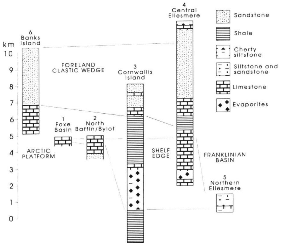
**Figure 9** Generalized stratigraphic columns showing thickness variations and geologic correlations of early Paleozoic strata across the Arctic Platform and into the Franklinian Basin. A thick foreland wedge of late Paleozoic age covers most of the northern Arctic Islands. Lines of correlation are time lines derived from biostratigraphy (after Trettin, 1991b).
