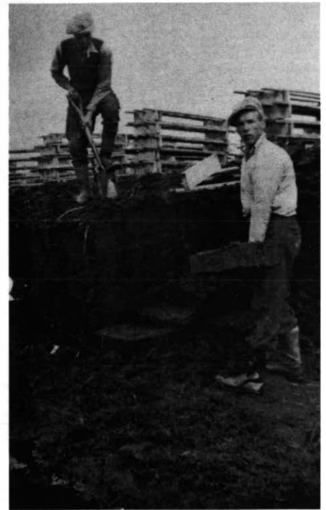
Figure 5 Cutting peat by hand in 1940s, Rivière-du-Loup, Quebec (Archives of Ministère des Ressources naturelles, Quebec).
