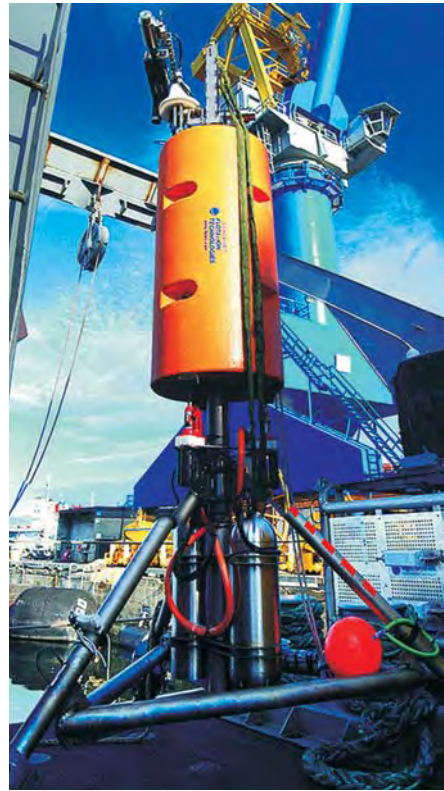
Figure 7. COVIS multibeam sonar, used to obtain 3D images of 3D hydrothermal vent fluxes, prior to deployment at the Endeavour Segment of the Juan de Fuca Ridge (2300 m water depth).
