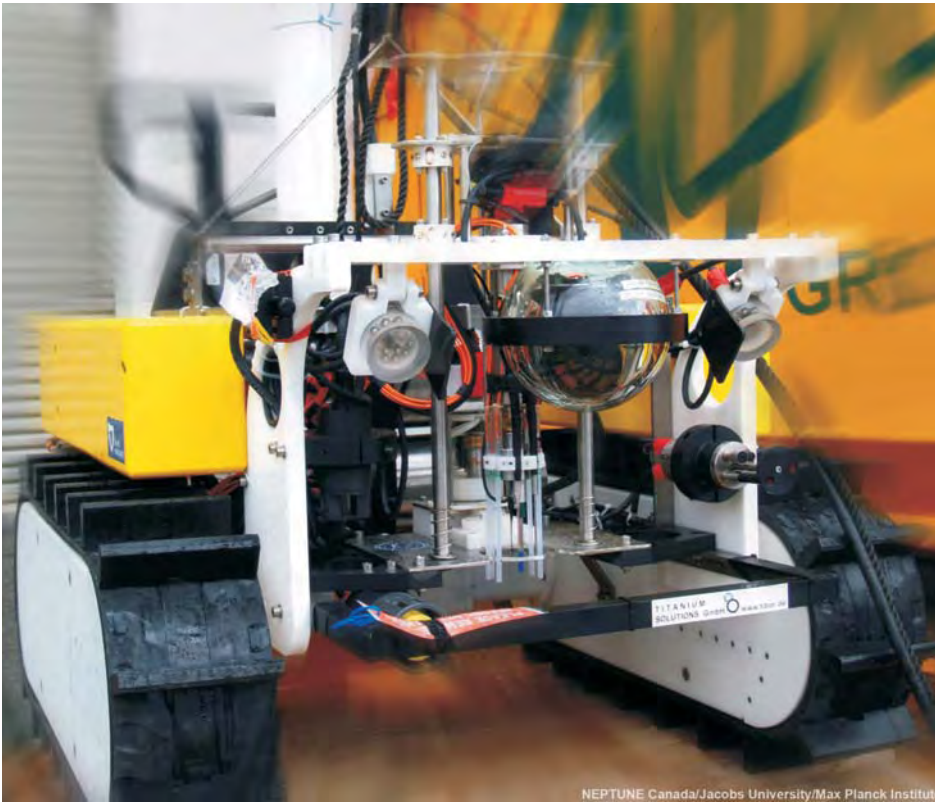
Figure 3. Wally II, the crawler from Jacobs University, Bremen, being tested at the Marine Technology Centre prior to deployment at Barkley Canyon (900-m water depth).
