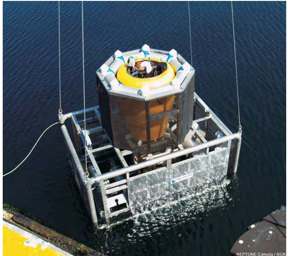
Figure 2. Deployment of the 2-tonne Vertical Profiling System, near Barkley Canyon (400 m water depth).
