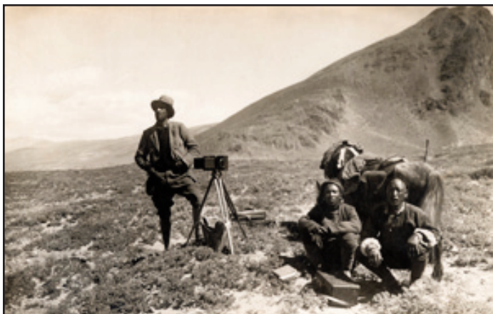
Figure 5. E.O. Wheeler and two of his three Tibetan assistants: Gorang, Lagay and Ang Pasang. Using a Canadian-designed photo-topographical survey camera with 12 x 17 cm plates, Wheeler took 240 single images and panoramas of the northern, western and eastern approaches to Everest, from which the first accurate topographical map of the area was constructed (Fig. 6). The technique required clear and relatively calm conditions, seldom encountered at elevations above 5000 m (wrt sea level) where the team worked for long periods. Photograph in 1921 by Sandy Wolaston courtesy of the Royal Geographical Society.
