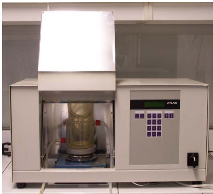
Figure 2. CPS+ ATLAS Suntest simulator. Simulateur solaire CPS+ ATLAS Suntest.
