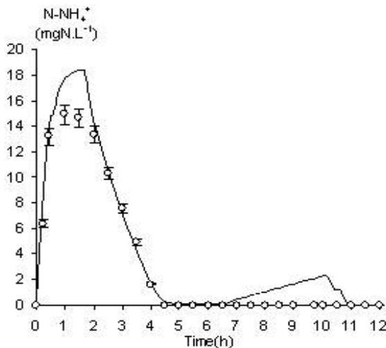
**Figure 4.** Correlation between model and experiment for  $\text{N-NH}_4^+$  during a pilot scale cycle.
