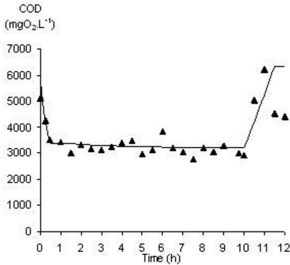
**Figure 3.** Correlation between model and experiment for COD during a pilot scale cycle.
