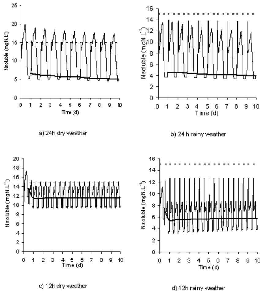
**Figure 2.** Evolution of the soluble Nitrogen concentrations during the simulations over ten days for the 24-h and the 12-h cycles (dry and rainy weathers). The continuous lines represent the exit concentration evolutions of soluble nitrogen at the end of the cycle, just before the discharge; the broken line represents the French standards required for the exit water.
